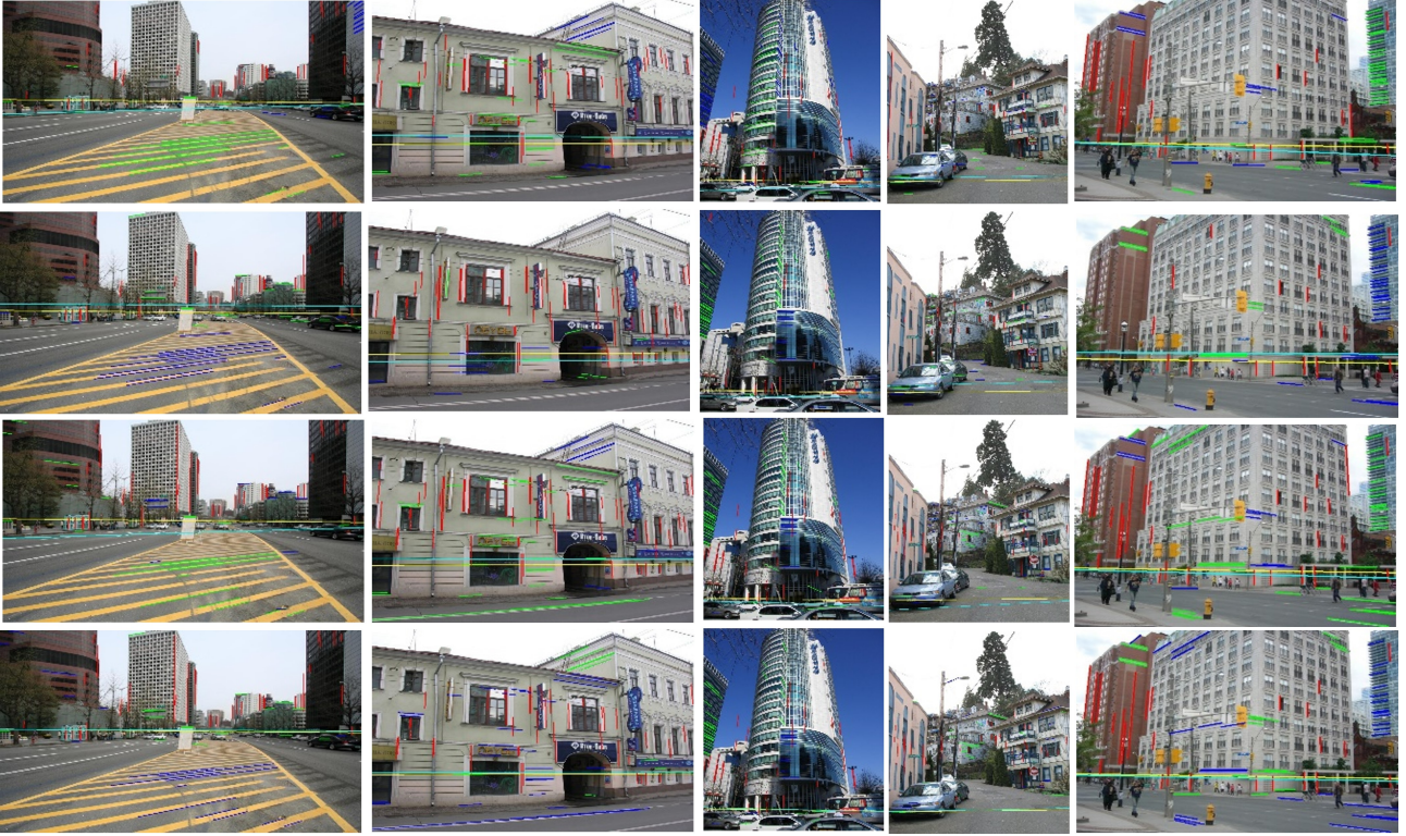
Fig. 13. Examples of all methods. The first row images are prev. work, the second row images are our, the third row images are R4L_MLE_Rf , and fourth row images are our_opt . The yellow line is the horizontal line of ground truth, and the cyan line is the estimated horizontal line.
